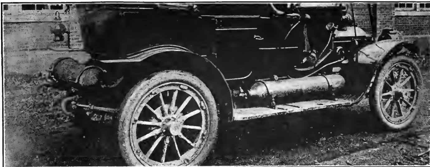
Packard car, showing mounting of the compression tank containing the liquefied natural gas which is used as fuel
